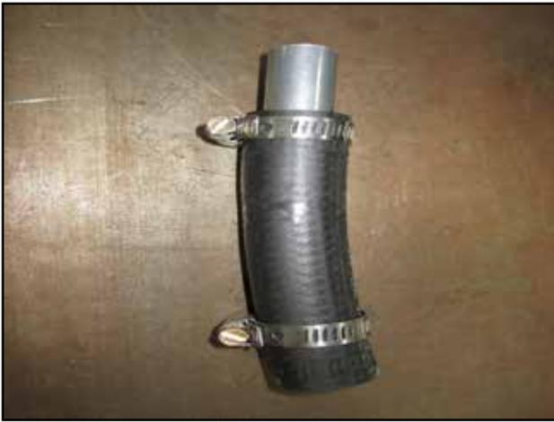
l. Insert nipple (8) into hose (7) and use the two (9) hose clamps on the hose as shown. Tighten the hose clamp on the nipple.
