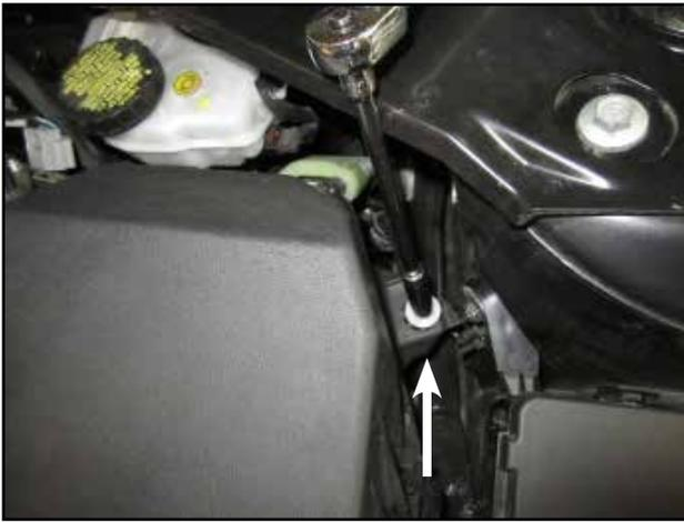
e. Remove the M6 bolt from the lower airbox.
