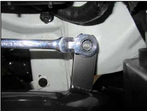
p. Now tighten the M6 (11) nut on the intake tube bracket.
